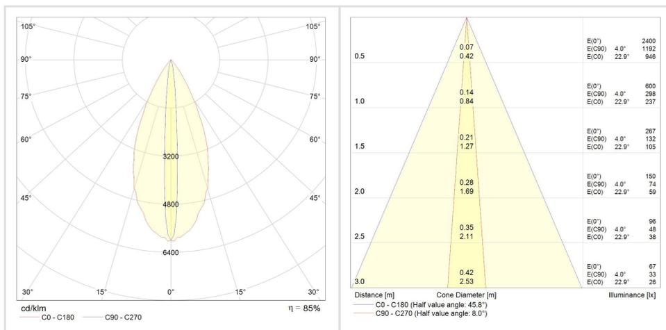
Lighting data referenced to 100lm CREE XP-E led flow.
